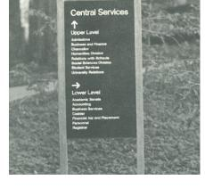
**Original:** The signs are fabricated from plastic laminate and are wall-mounted or supported by redwood posts. The type is silk-screened directly onto the plastic laminate surface and can be removed with the use of paint thinner for alterations.
