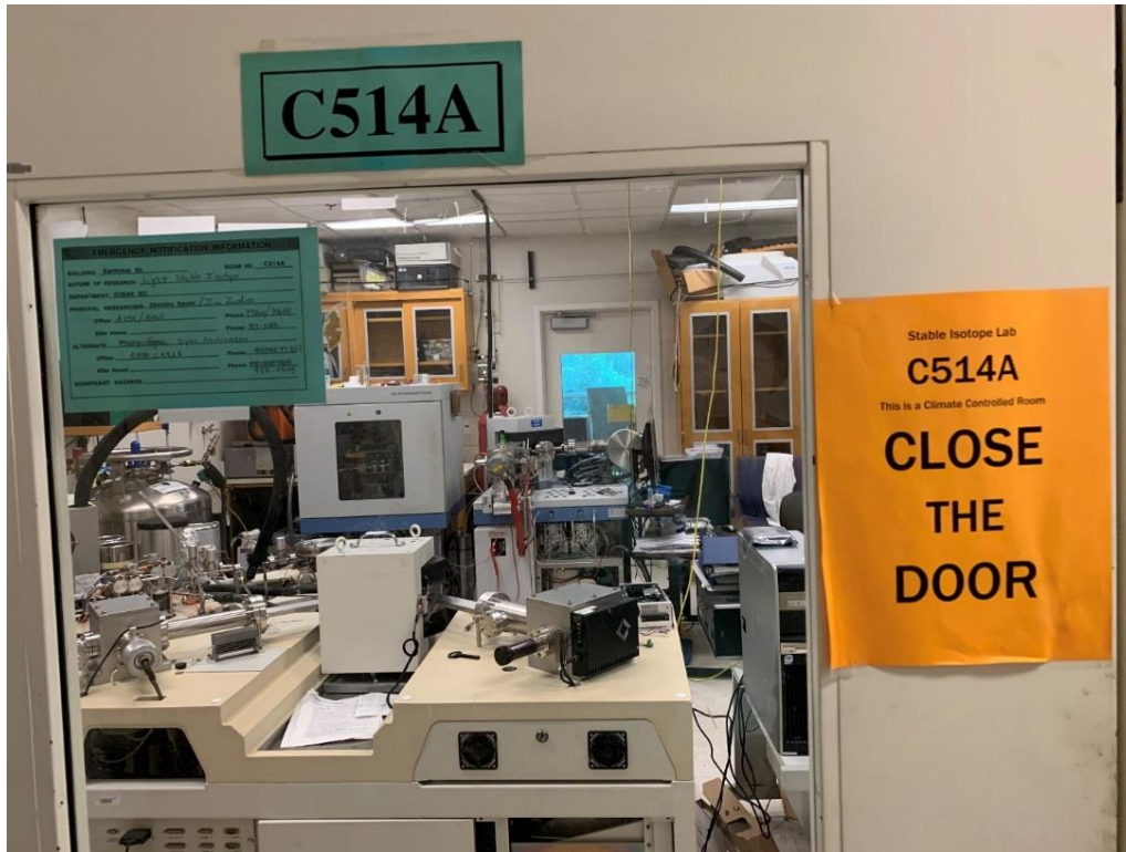
Building C Room C514A Unanchored Laboratory Equipment
