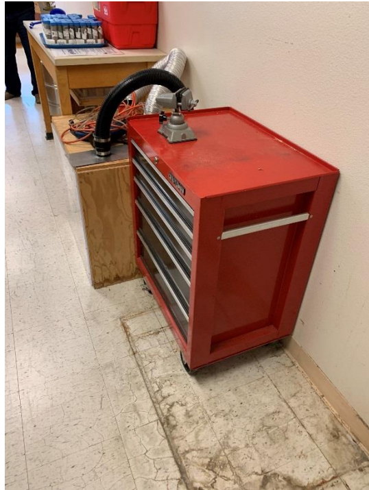
Building C Room C514 Toolbox Unanchored
