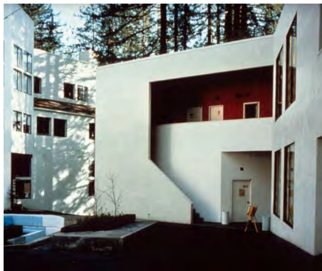
Fig. 4.1.3-1 Accent color on underside of balconies, stairs, walkways, ramps, interior face of screen walls, recessed entries (Kresge College, Morely Baer Photographs - UCSC) Archives)
